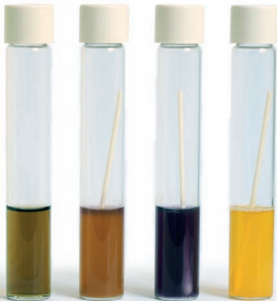
RV-Broth was inoculated with 1 µl of an overnight culture and incubated aerobically for 24 hours at 36°C – from the left: 1. negative control 2. Enterobacter faecalis WDCM 00009 3. Pseudomonas aeruginosa WDCM 00024 4. Escherichia coli WDCM 00012
