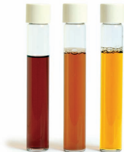
BfW-Broth for Wildtype Yeasts with indicator For the realistic implementation of the analysis, 1 ml of hopped beer was first added to the broth and only then was inoculated with the yeast strains. The incubation was carried out aerobically for 6 days at 25°C ( B. bruxellensis ) and 2 days at 25°C (Wildtype strain) – from the left: 1. negative control 2. Brettanomyces bruxellensis DSM 70001 3. Wildtype yeast from young wine
